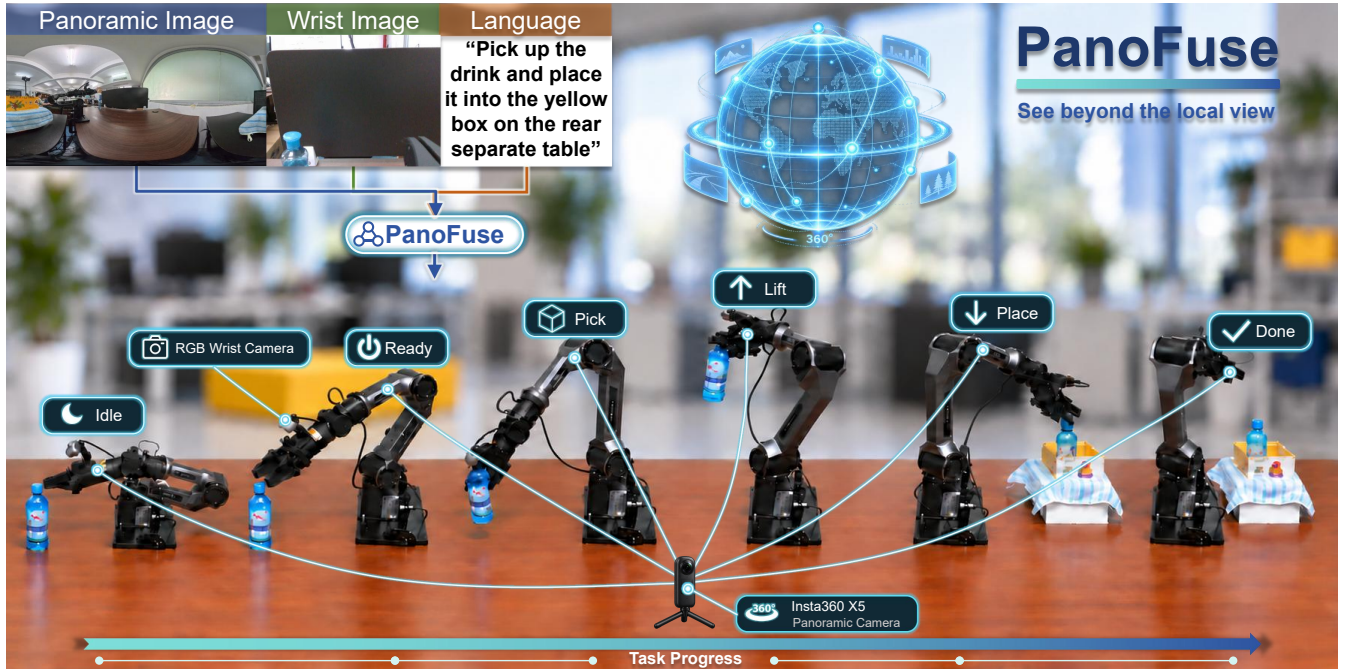
Fig. 1: Overview of PanoFuse for real-world robotic manipulation. PanoFuse complements local wrist-camera observations with a 360° panoramic view to provide global scene context. The illustration shows a representative long-horizon manipulation sequence, where panoramic perception supports continuous action generation from target acquisition and grasping to transfer and place.
