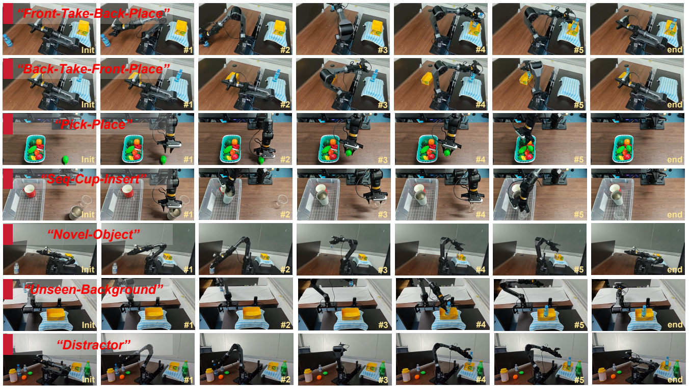
Fig. 4: Representative real-world closed-loop rollouts of PanoFuse across seven evaluation settings. PanoFuse leverages panoramic semantic and geometric context for global scene understanding and task-relevant spatial reasoning, enabling robust manipulation under cross-workspace, novel-object, unseen-background, and distractor-rich scenarios.
